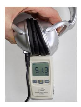
Verify in the setup that continuous tone, long enough, eg 5000 msec is selected. Place the meter between the headphone as above.
